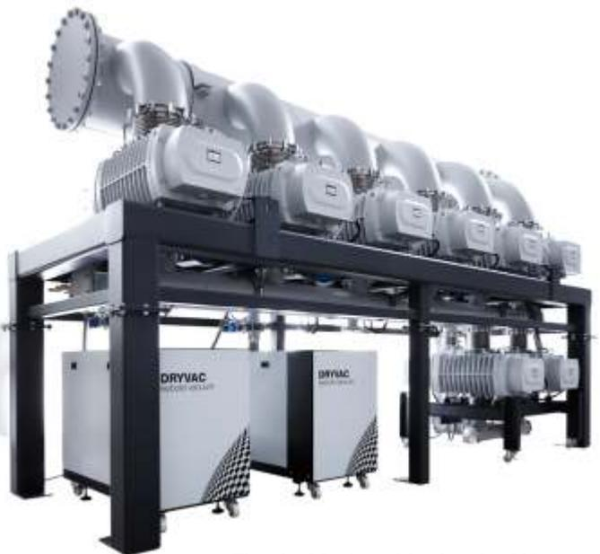
Fig. 1 : Modern Mechanical Vacuum System for Steel Degassing
