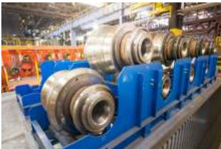
**A**rcelorMittal Belval, based in Esch-sur-Alzette, Luxembourg, has started up the CRS® Compact Roller Straightener supplied by SMS group. It only took four-and-a-half weeks to dismantle the previous equipment and install the new straightener, including successful commissioning. The new straightener can handle the largest sheet piles currently produced in the world, expanding the range of products producible at Esch-sur-Alzette.
