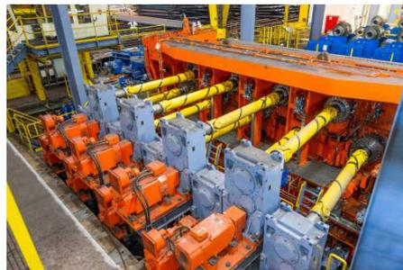
Z-type and U-type sheet piles as well as flat sheet piles. Equipped with double supported design instead of the conventional cantilever design, the machine provides for a balanced force distribution, leading to better straightening results especially for extra wide sheet piles.
