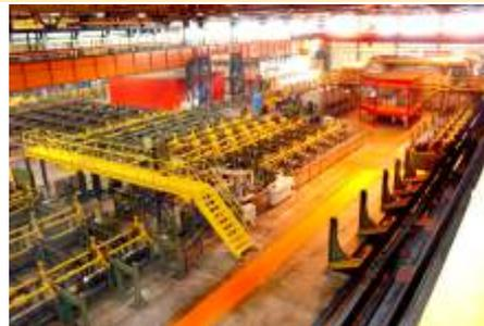
furnace with walking beam transport system, a quenching head, a quenching tank, a walking beam tempering furnace and a cooling bed. The line allows carrying out various process steps, such as quenching, tempering and normalizing.
