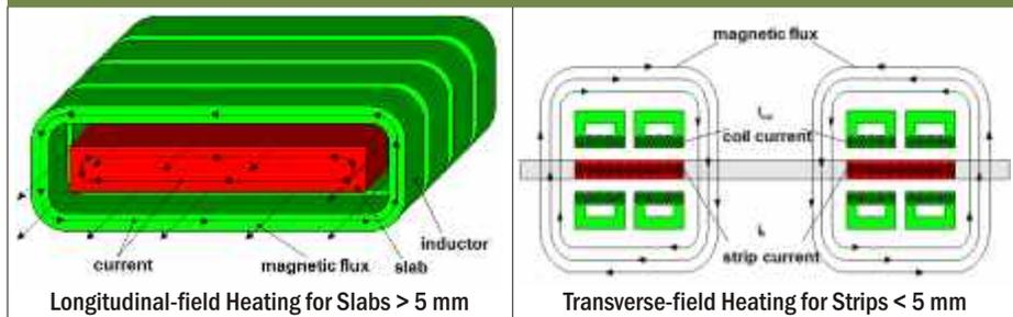
**Basic Configuration of an Induction Heating Unit In A Rolling Mill**
