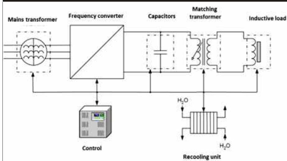
transformer is to transform the mains voltage into the operating voltage of the frequency converter. The mains transformer acts as the link between the customer's mains power supply and the induction heating unit. The voltage supplied by the mains transformer is a 3-phase AC voltage. By the frequency converter this AC voltage is first transformed into DC voltage, and then converted into single-phase AC voltage with the required operating frequency.
