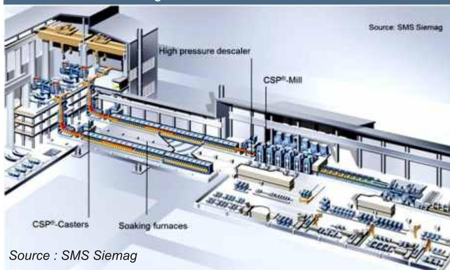
in the line where a temperature increase is required – for example at the inlet or outlet of the roller hearth furnace, between the roughing stand and the first finishing stand of the mill, or between the last finishing stands.
