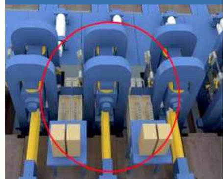
In the endless rolling process for very thin strip grades or silicon steels, compact, integrated induction units between the finishing stands compensate the temperature loss and guarantee the right temperature level at the end of the finishing mill.
