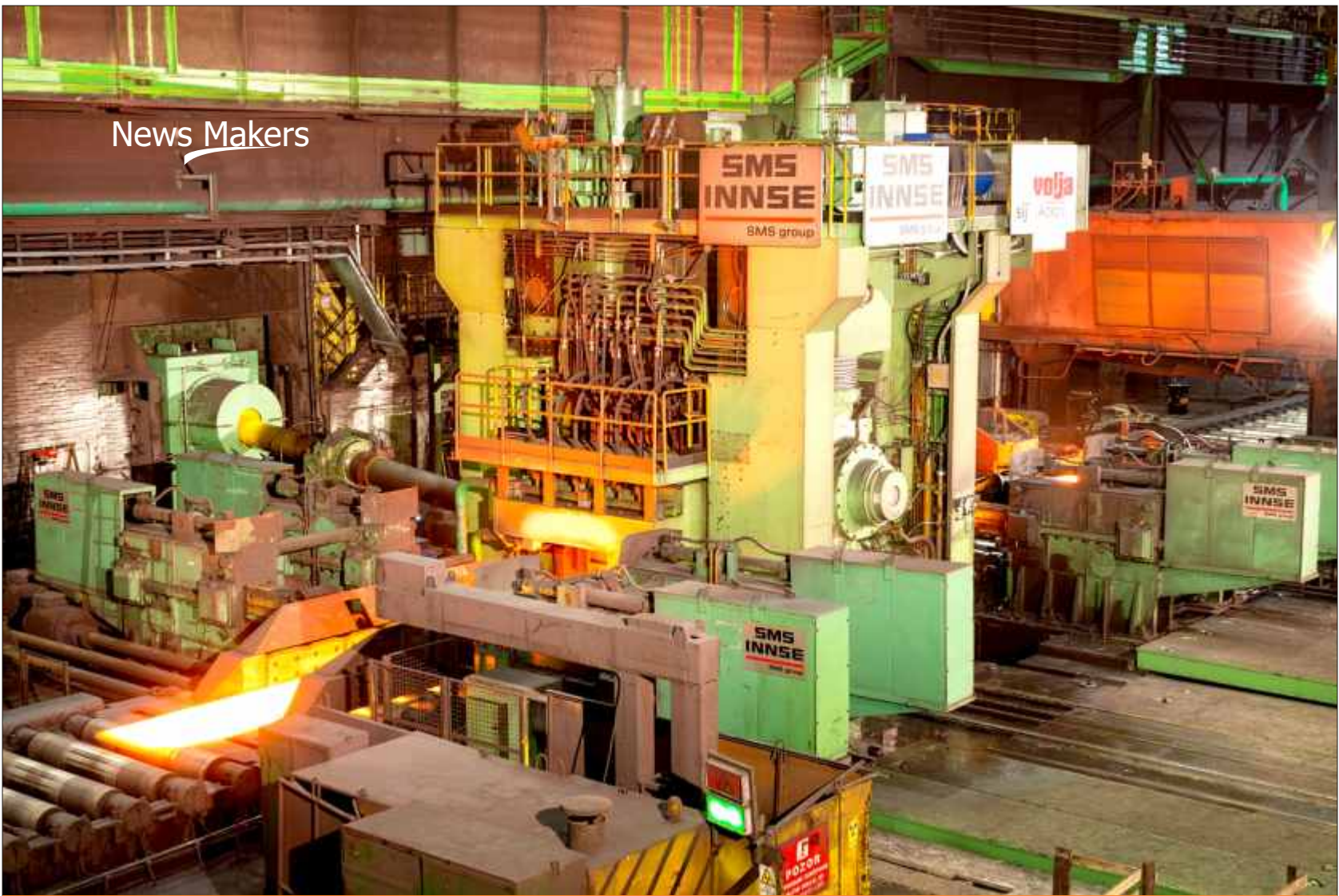
The New 2.6-m Heavy-plate Mill Stand of the Slovenian Steelmaker Acroni
