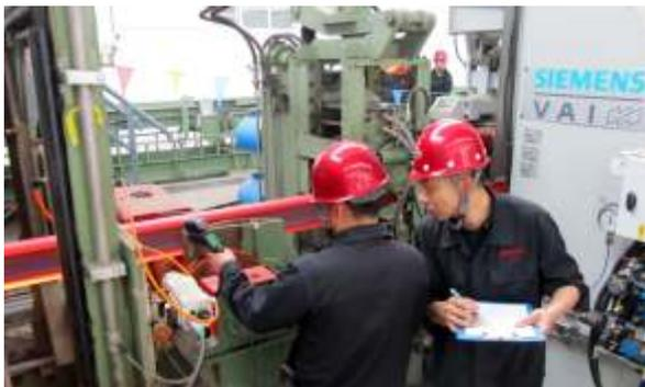
Brinell HBW10/3000 at the surface of the rail head, and from 34 to 42 Rockwell HRC across the rail section, according to the applicable measuring protocol. R60 U75V gr.340 is the first rail in the world to be commercially processed through Idrha+, and is now in industrial production already at a rate of 15 pieces per hour with a 100 m standard length.
