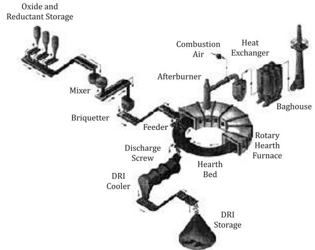
slag separates from the metal. The metal nuggets and the slag granules can be easily separated post cooling using a screen or a magnetic separator. The iron nugget usually contains about 3.5% dissolved carbon. The nuggets can be directly fed into a BOF or an EAF. The schematic of the process is given in Figure 8.
