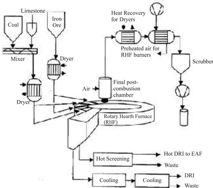
are fed as a mixture in this case. The residence time is similar to the COMET process. Due to the higher residence time, the productivity of this process usually remains lower than the pellet based processes. The DRI is then melted in a separate electric arc furnace like in the other processes. Figure 6 shows the process flow diagram of this process.
