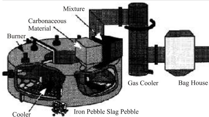
preheating zone in order to extract the maximum chemical energy stored in the burner fuel. Elimination of entrapped moisture and the volatile matters take place in this zone.
