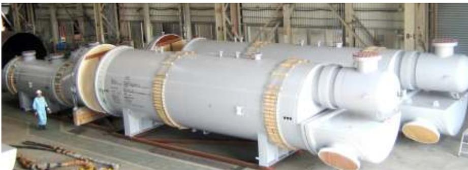
**K**obe Steel, Ltd. has announced that its intermediate fluid LNG vaporizers (IFVs) will be used in the regasification facility for the Delimara LNG Regasification Terminal under construction in Malta. Kobe Steel will supply two IFVs. Each unit will have a regasification capacity of 58 tonnes per hour. Kobe Steel plans to ship the IFVs in October 2015.
