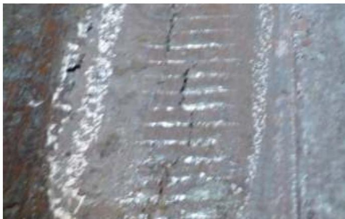
Figure 1 : Web Surface Cracks on Beam Blank
