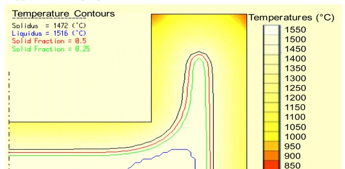
Figure 3 : Existing Temperature Profile of Simplified Beam Blank Geometry Quarter Cross Section at 2 M Below Meniscus of C18 Grade for Small Beam Blank at 1.1 M/min
