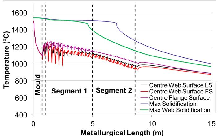
During a plant visit the simulated surface temperatures on all faces have been verified with pyrometer measurements at the caster. Based on these results an optimised secondary cooling system was designed maintaining good quality at increased speeds and productivity. The water supply was to remain as existing, for segments 1 and 2 additional air-supply had to be proposed.
