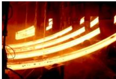
This is a combination of high speed caster to produce billets and blooms in square and round sections. It has 8 strands and is the largest and first of its kind in the world. The nominal capacity of the machine is 2 MTPA. The machine is capable of casting the following range of sections.
