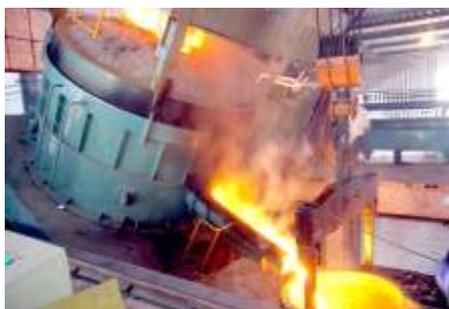
With nominal capacity of 200 tonnes, this is the largest in Middle East. It has unique feature to directly charge Hot DRI at 6500 C into EAF by gravity and thereby facilitates substantial energy saving. This is the world's first gravity hot DRI feeding system. The furnace is modern and technically superior.
