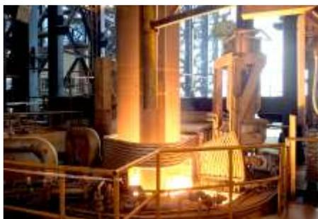
Capacity of the furnace is 200 tonnes. This is one of its kind in Middle East. Liquid steel is treated in the furnace to get desired chemistry and temperature.
