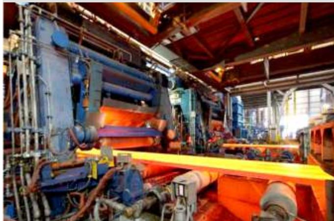
Benxi Iron & Steel plant (P.R. China), pioneering silicon steel production in China using Thin Slab Casting technology, which successfully cast silicon grades with a Si content up to 3.2% at over 4 m/min.
