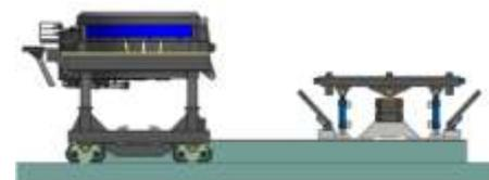
In order to prepare the furnace for restart, the shell can be loaded with remaining liquid steel or scrap prior moving to the operating position.
