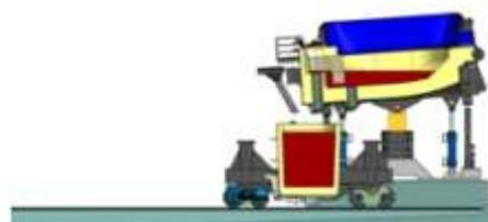
with cylinders and guides, allowing the shell to be tilted in both directions – tapping and slag side.
