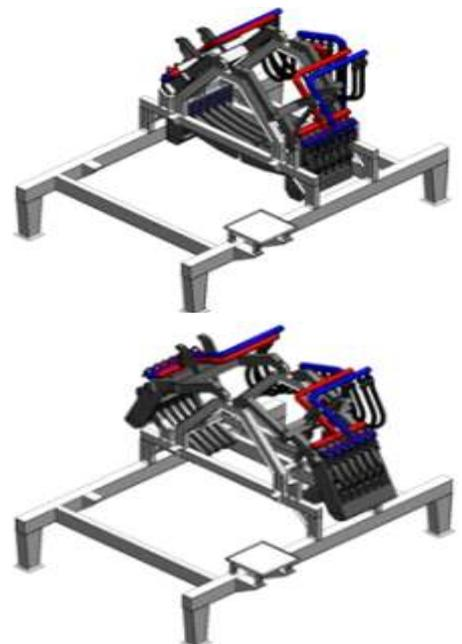
fingers can be closed immediately afterwards for loading and preheating the next batch of scrap. All this can be done under power-on.
