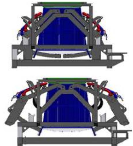
**FIGURE 5 : SCRAP RETAINING SYSTEM ON MAIN FRAME IN CLOSED AND OPEN POSITION**
