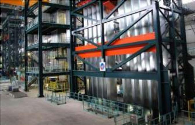
Russian steelmaker PAO Severstal awarded CMI Industry Metals the design and supply of a hot-dip galvanizing line (HDGL) and a color coating line (CCL) for its Cherepovets steel mill. These high-capacity lines will produce 400,000 tpy and 200,000 tpy and reach process speeds of 180 m/min and 120 m/min respectively. They will be commissioned by April 2017.
