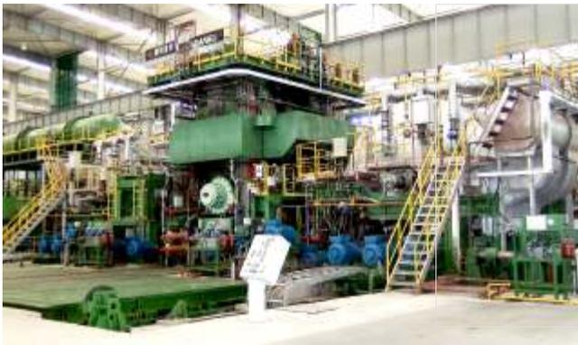
The Chinalco Steckel mill plant was designed to produce 4,000 tpy of plates and 58,000 tpy of coils for stainless and non-ferrous alloys (titanium, nickel and copper) for a total capacity of 62,000 tpy. Thanks to its compact design, a complete line from cast ingot furnaces to plate finishing line can fit into only 200 m.
