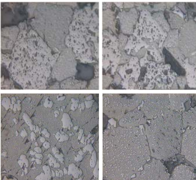
FIG. 1 X 2000 BRICK A REBONDED FUSED GRAIN
