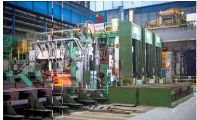
conventional casting and rolling mills. Energy consumption is up to 45 percent lower than in a conventional casting and rolling process, and CO2 emissions are also significantly lower.
