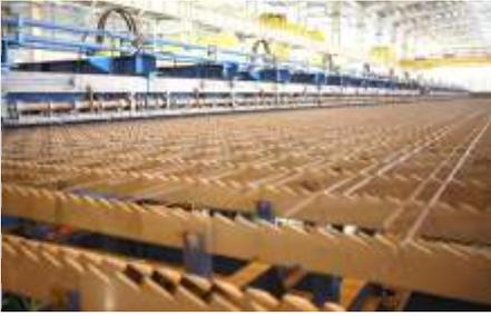
**H**TC technology is the way to obtain high productivity with small size bars, delivered at ultra-high speeds onto the cooling bed, one bar per notch, both for one-strand and two-strand rolling.
