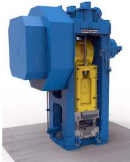
electric walking beam type EHA of SMS group comprising four individual housings with the drive fastened to the outside of the press frame, thus ensuring that contamination from scale and dirt is prevented. The automatic system guarantees a finely balanced and smooth motion. To achieve this, EHA features a separate drive consisting of servo motors with dedicated gearing for each axis. The three axes of motion of the
