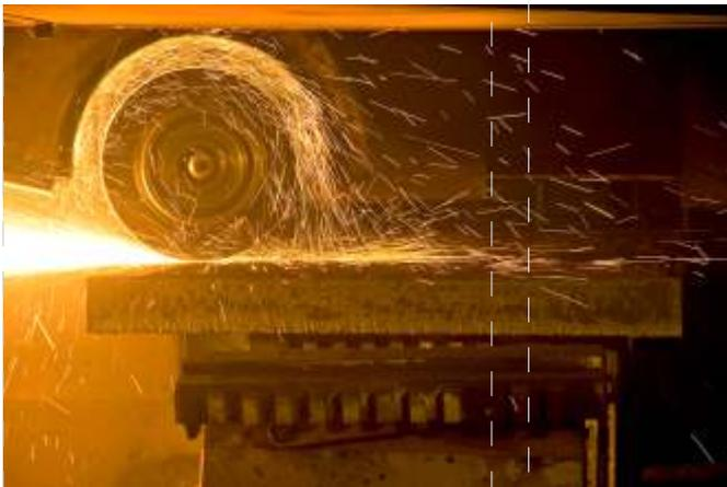
Baosteel and Danieli jointly completed the performance tests on the new Baoshan Inspection and Grinding Plant which is now in production. The new concept is based on the integration of scarfing for primary conditioning (full skin) and grinding for secondary conditioning (spot or pattern removal) in order to deal with large volume of carbonsteel slabs, over 1.2 MT per annum. This process method allows to drop the volume of removed steel to the very
