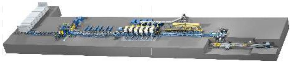
high reversing roughing stand with edger, the six-stand finishing mill, a laminar strip cooling section, a universal coiler and the coil transfer system. At a later stage, the annual production can be increased to upto 4.0 million tons per year.
