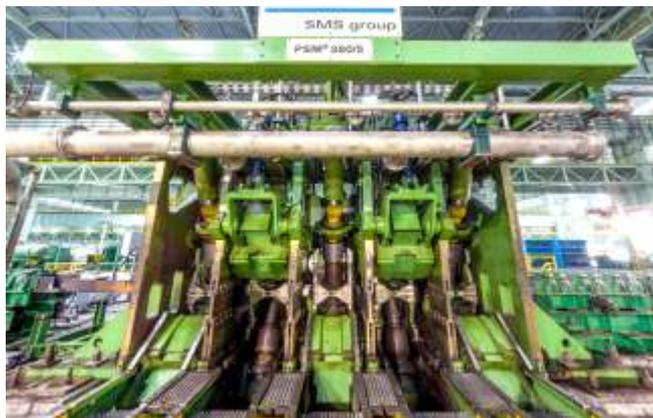
The Chinese company Qingdao Iron and Steel from Qingdao, Shandong Province has awarded SMS Group the FAC for the supplied SBQ (Special Bar Quality) mill. After a short ramp-up phase, the new special mill is now producing a wide range of steel grades with very good mechanical properties and optimized microstructure with tolerances of better than 1/6 DIN. The mill is designed for an annual capacity of around 700,000 tons of bar steel.
