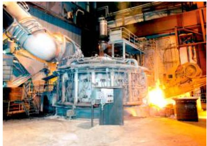
weight of 140 tons, an installed power of 130 MVA and is equipped with the pin-type bottom electrode patented by SMS group. The revamp took place during the shutdown in summer 2016.
