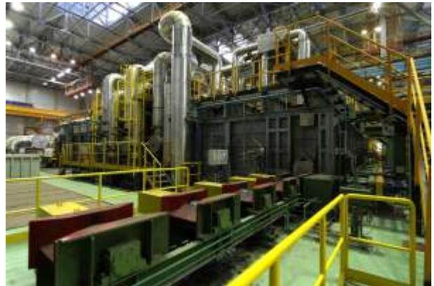
millimeter square billets with a length of 12 meters and 300 x 250 millimeter beam blanks, heated in a walking beam type reheating furnace.
