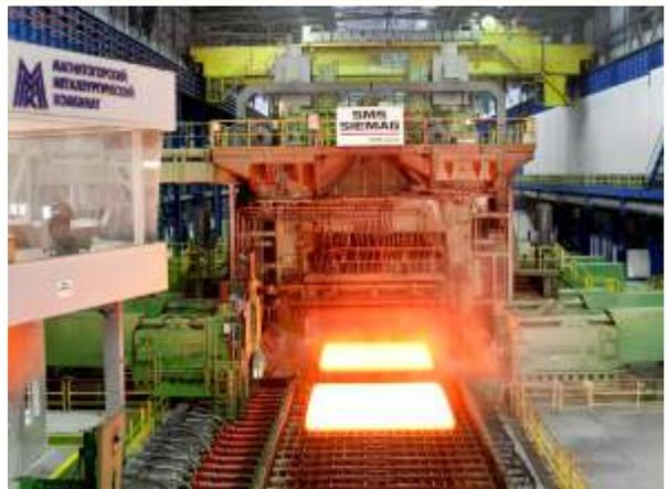
millimeters. This will be achieved mainly by modifying the CVC roll bending and shifting system, installing new chocks for the upper work roll and adapting the back-up roll balancing system. SMS group will also supply a new level-2 model for the reheating furnaces and an upgrade of the process models in the rolling mill.
