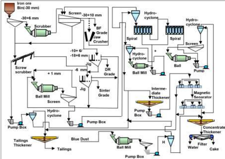
**Fig.5 Process flowsheet for physical beneficiation of low grade ores**
