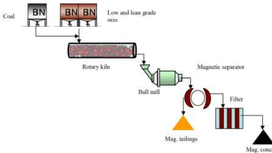
**Fig.8 Schematic diagram of reduction roasting process for iron ore**
