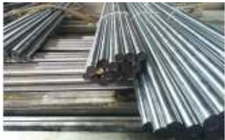
Dalian Special Steel trial produces the new type cold work die steel D2S successfully. The steel is Cr8 type cold work die steel designed by the custom, the composition is new designed,
