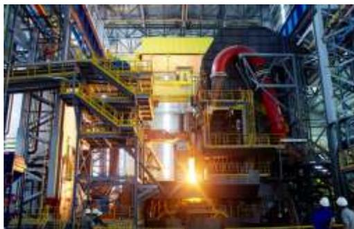
complete mechanical and electrical process equipment and the automation technology. This includes the automated scrap yard management, the automated charging process, automation of the oxygen injection and sand refilling, as well as the Level 2 automation which makes the plant ready for Industry 4.0.
