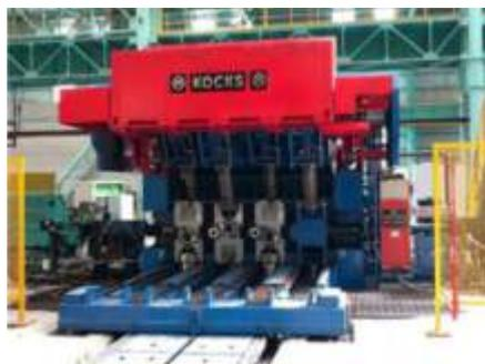
Maanshan Iron & Steel Co., Ltd. (Masteel) has successful commissioned the new small bar mill incorporating a Reducing & Sizing Block (RSB®) 370++/4 in 5.0 design by Friedrich KOCKS GmbH & Co KG. The
