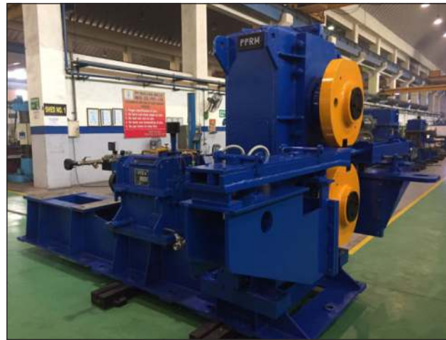
Combination Shear to cut 8 mm to 40mm with 8mm @ 40mps and 40mm @ 2mps
