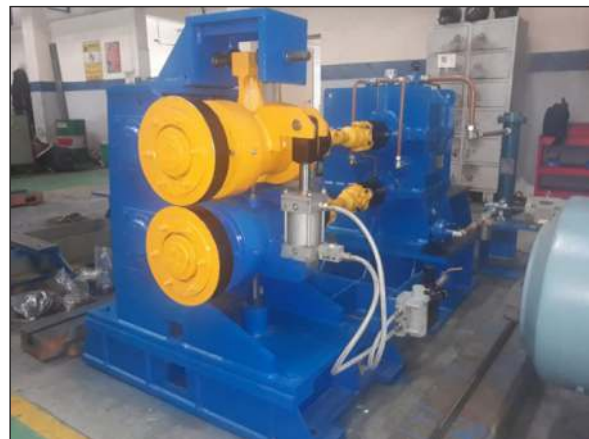
High Speed Pinch Roll @ 30 mps
