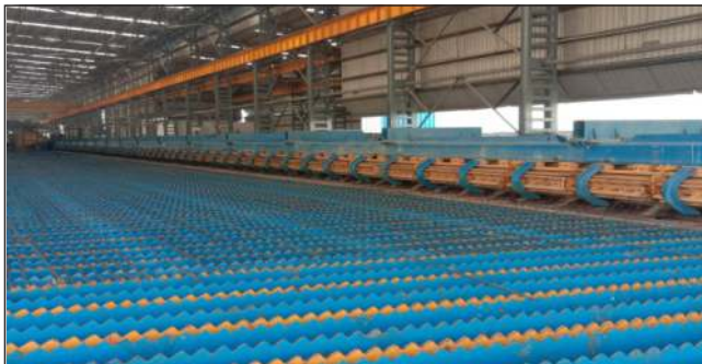
High Speed Rotating Drums can handle 8mm Rebars at 40 mps
