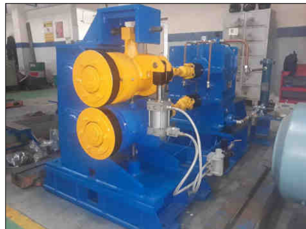
High Speed Pinch Roll @ 30 mps
