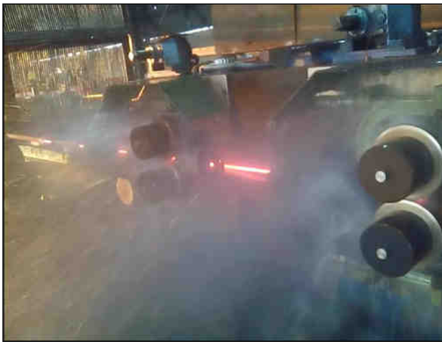
Cantilever Stands for TMT Bar from TC Rings with groove life of 800-1000 Tons @ 24 mps
