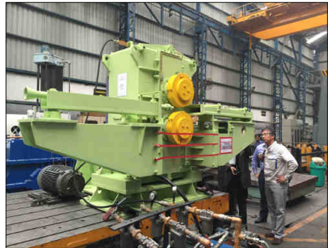
Continuous Operating Shear to cut 8mm rebar to 16mm in High Speed exported to KOBELCO Japan
