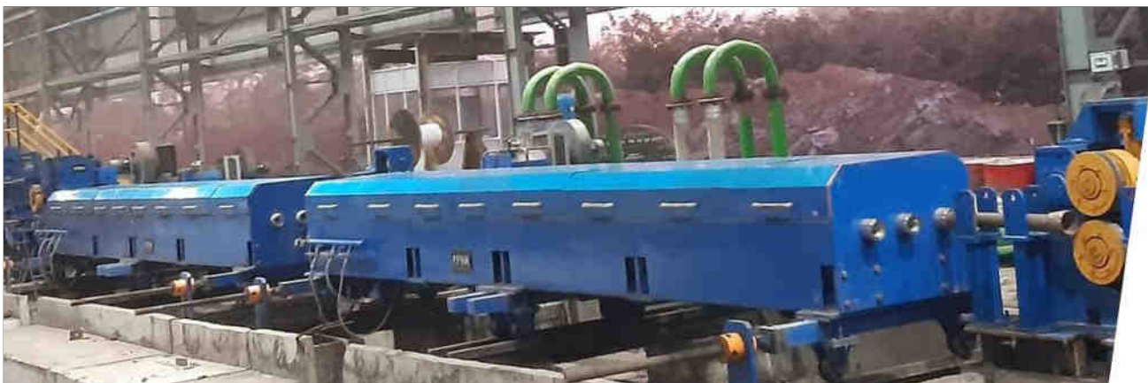
High Speed Quenching Lines
